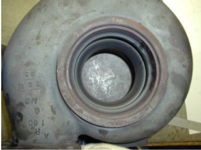
Figure 20: Volute of New Turbine Housing Design After 500 hours of Gas Stand Endurance Testing.
