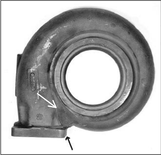
Figure 1: Volute Crack on A Hosing Subjected to Aggressive Field Duty Cycle
