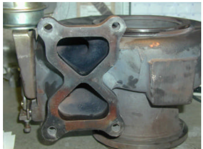
Figure 19: Inlet Flange of New Turbine Housing Design After 700 hours of Gas Stand Endurance Testing.
