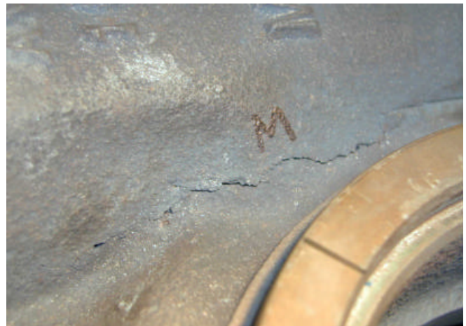
Figure 15: Baseline Turbine Housing Cracking at Volute after 200 Hours of Gas Stand Endurance Testing.
