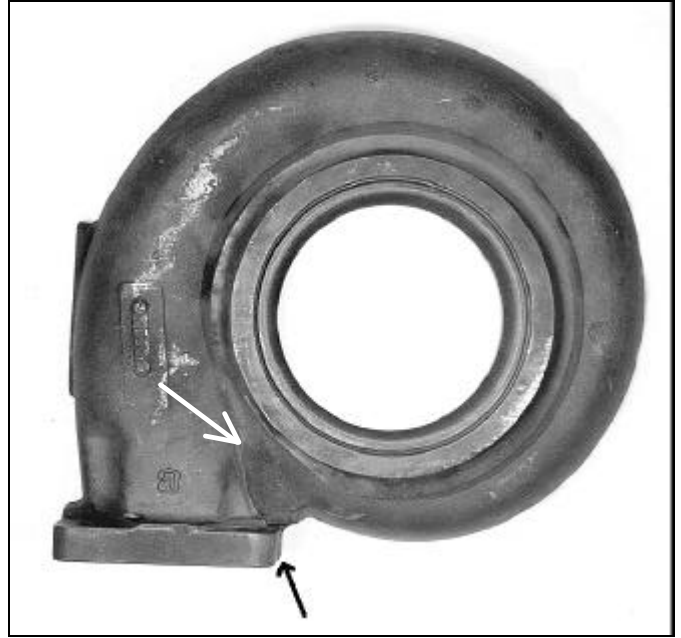
Figure 1: External Volute Crack of A Dual Entry Housing.
