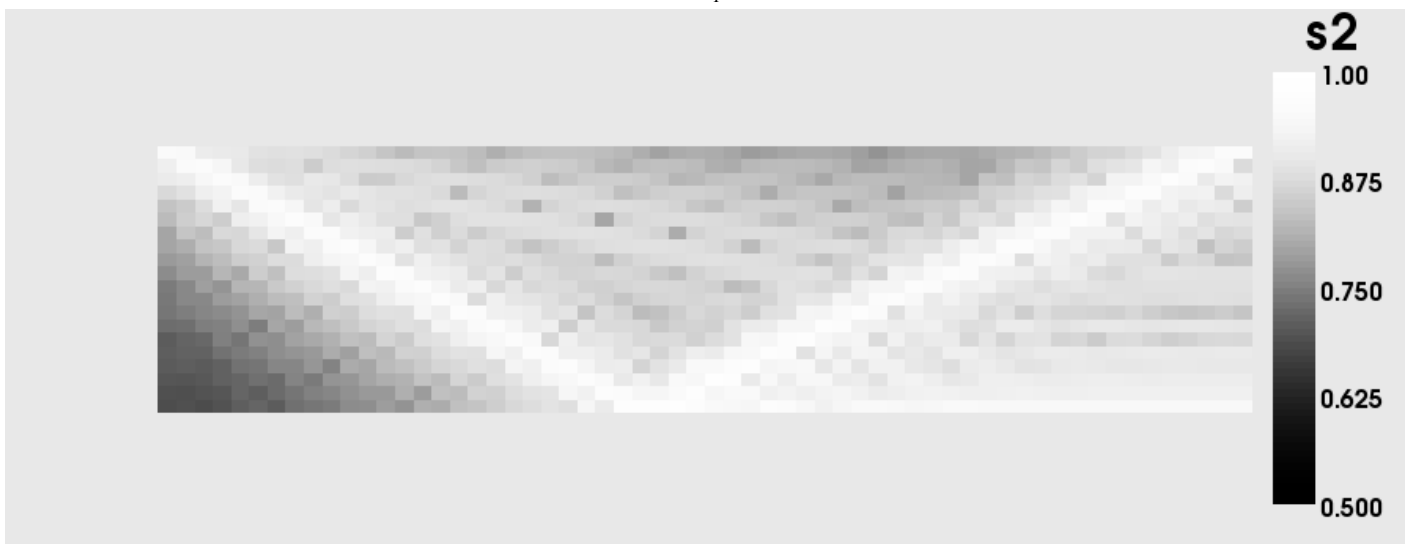
Figure 6 The second order implicitness parameter s_2 contours for shock-reflection test case, 60x20
