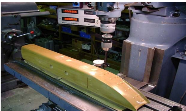
Figure 2. Picture of train model displaying longitudinal fins.
