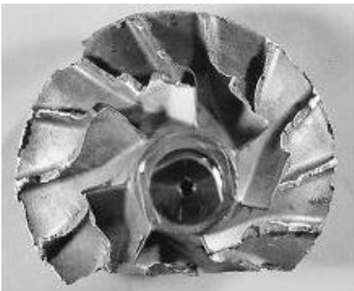
Figure 2 – Back disc failure in compressor wheel
