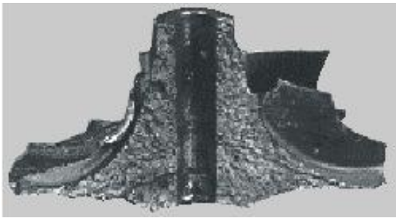
Figure 1 – Hub failure in compressor wheel
